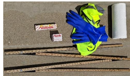
Stick for fuel gauging, fuel-finding paste, and other equipment
