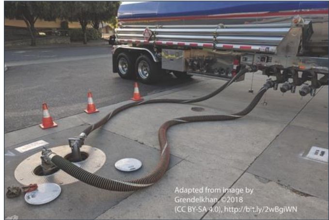
Product delivery using Stage I vapor recovery
